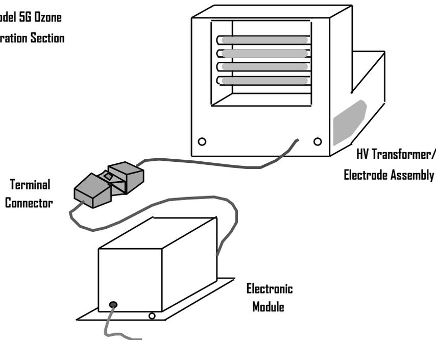
Unplug the power cord for the 5G. Field testing of the electronic module will require a digital voltmeter with ranges of minimum 300VAC. Initially verify that the electronic module (4) is getting power to it. Use an AC voltmeter to read the voltage on the airflow switch (28) with the blue wire. With the unit operating, activate the airflow switch and the blue wire terminal voltage should be line voltage (120VAC or 240VAC) according to the voltage level of the unit.
